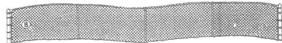
B Fence following grade, rolling terrain
